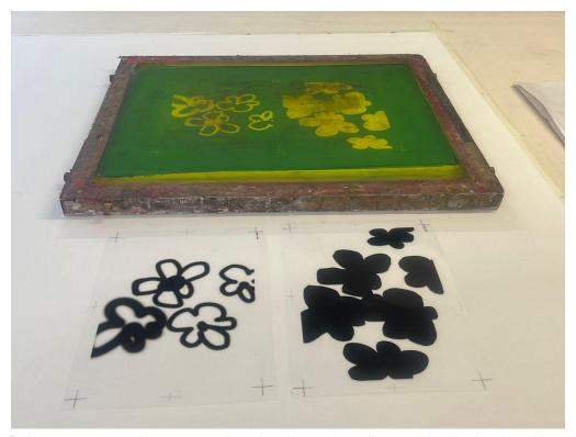
Below you can see the two artworks printed out; the outline and the block colour. Here the screen has already been exposed with the designs.
